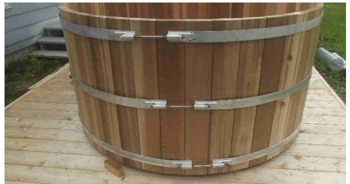
Fig. 8.1 Proper placements of straps and bolts. Note how bolts straddle a seam between staves and are staggered.
