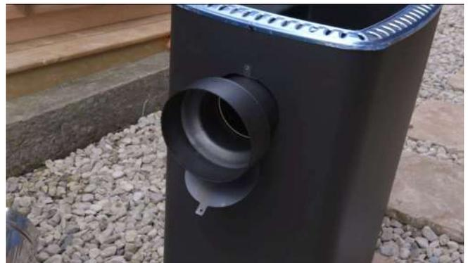
Install back wall shield centered over chimney hole with 1 ½" (38mm) screws.
