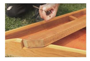
15. The beam will sit on an angle which should leave a gap underneath like in picture. Be sure to secure provided screws closer to where beam and roof panel meet.
